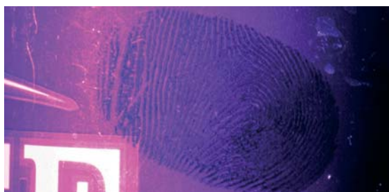
Photo 4: Bloodstained fingerprint. Obelux CR9, 417 nm, f 22, time 15 s.
